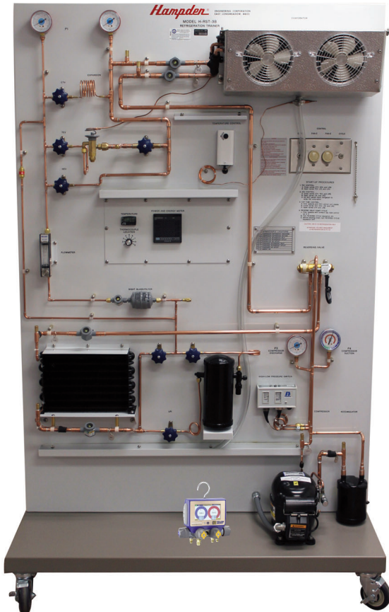
MODEL H-RST-3B shown with H-RST-DMP Digital Meter Package, H-RST-FP-10E/M Fault Package, and H-RST-TC Digital Temperature Package options (Shown with H-RST-DMB Option) Dimensions: 76"H x 51"W x 31"D Shipping Weight: 675 lbs
