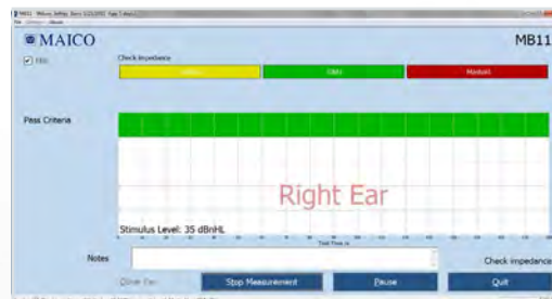
"Traffic light" display for electrode contact and test quality provides easy to understand feedback to screeners.
