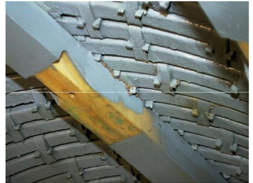
Insulation crack and abrasion between Endwinding and support elements
