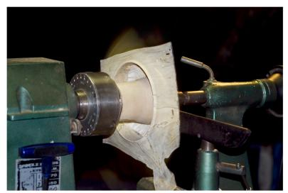
Using a jam chuck I reverse the bowl between centers using the original dimple on the base from when I rough turned the tenon on the log. I place a folded paper towel between the jam chuck and the bottom of the bowl, and move the bowl around a little until it runs true. Then cut off the tenon with light cuts, finish bottom detail as you like. See photo left and below left.
