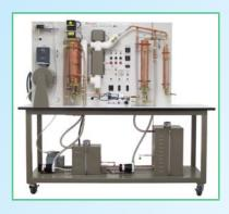
The Hampden **Model H-ETS-1A** Ethanol Production Process System is designed to facilitate the instruction of students on the process required to produce ethanol for experimental purposes. Ethanol is a very promising fuel alternative to oil since sources are widely available and ethanol is clean-burning. The student will be able to observe and control the process of producing
