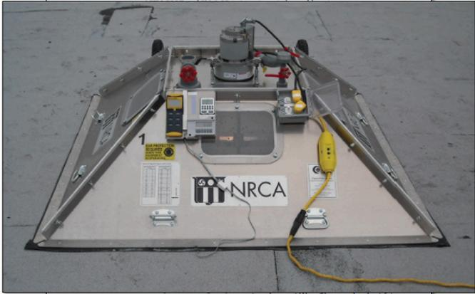
5-foot dome-like chamber to a roof surface's upside and applying a defined negative (uplift) pressure inside the chamber to the roof system's exterior-side surface using a vacuum pump (see photos). During the test, membrane surface deflection inside the chamber is visually monitored and measured to determine whether a roof system passes or is "suspect."
