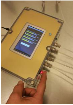
Step10-turn on pumps
