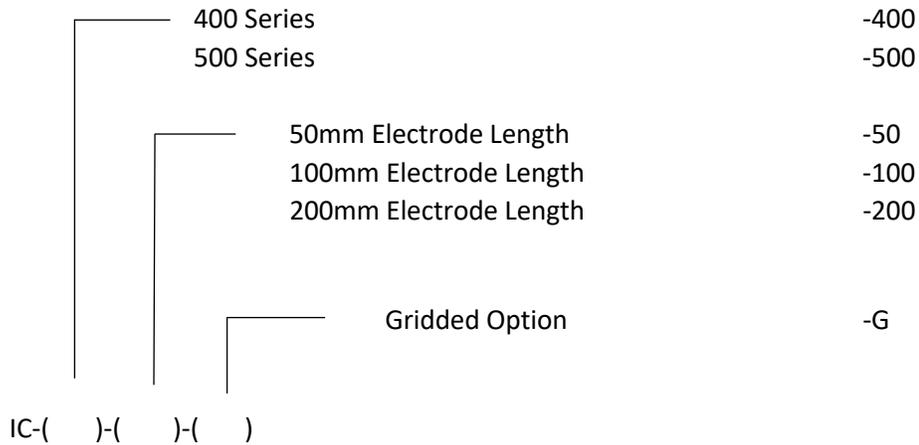
For example, an ion chamber 400 series with a 50mm Electrode length, with the gridded option would be denoted by: IC-400-50-G
