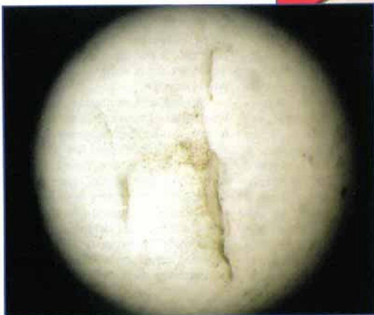
Photo 40 – Magnified view (10x) of top side of depression showing minor crack in membrane coating. (5)
