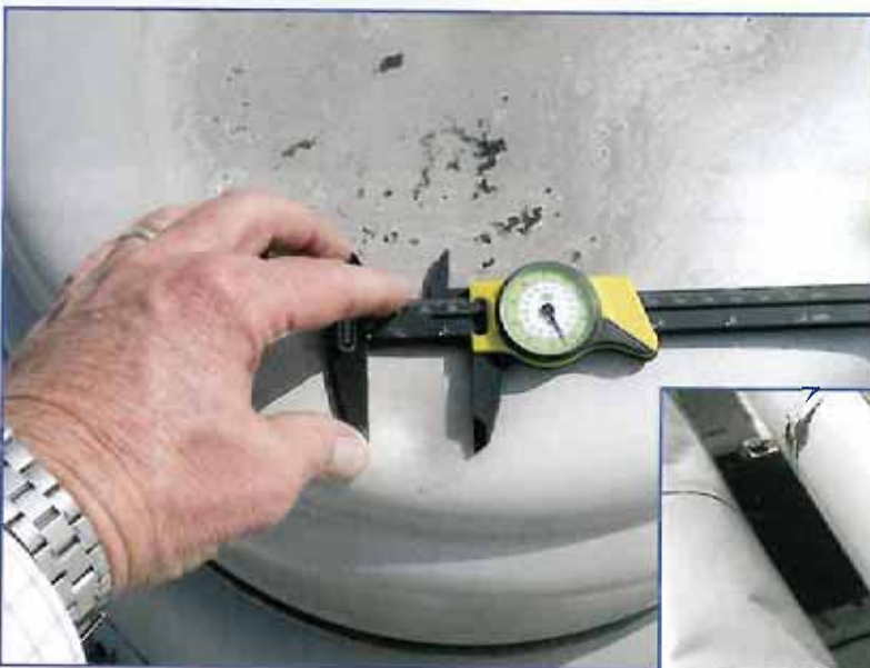
Photo 18 – Dents in metal equipment hood. (5)
