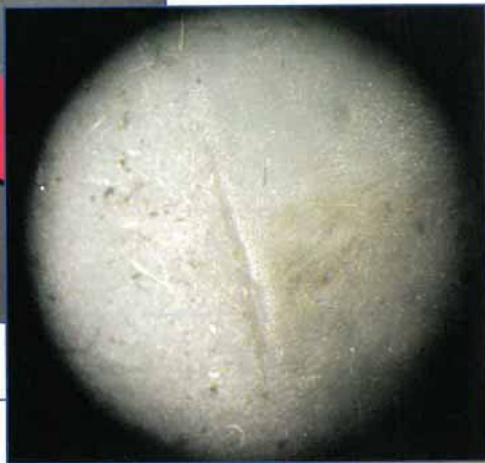
Photo 38 – Magnified view (10x) of depression showing minor crease in membrane. (5)
