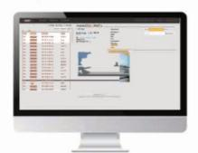
SmartMail was developed with the small/medium fleet operator in mind. It delivers driver safety and protection information to you within moments of an incident taking place. Using CP1 with a cellular modem, safety-critical road events will automatically transmit an email notification with the video clip and event information enclosed. An online portal is provided to help manage all vehicle events.
