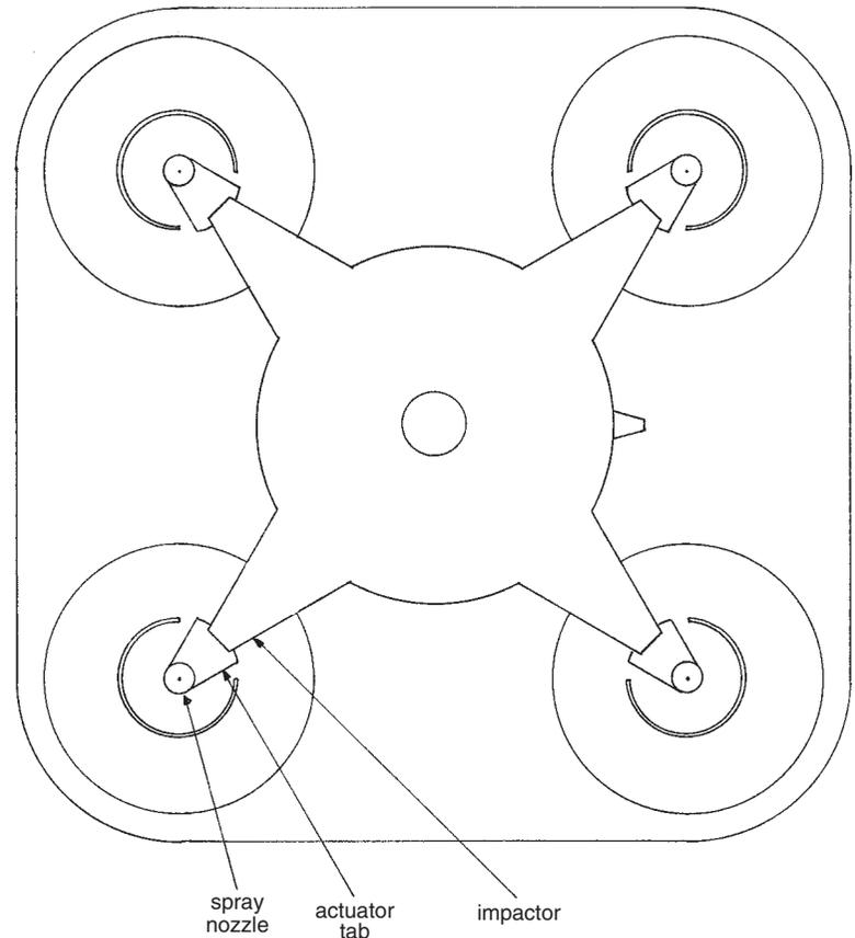
If in the future you wish to change the time setting it is not necessary to remove the cans. Just move the upper switch (1) to off. This disables the solenoids. As a further precaution you may wish to rotate the impactor part way out of position. The new time delay setting can now be checked by noting the duration of the warning horn. When resetting is complete slide the upper switch to on and rotate the impactor to its alignment position as shown in Figure 3.
