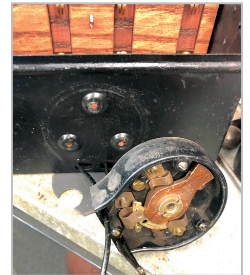
6) Lace new wires to the switch. Install gasket behind switch before fastening to coil box.
