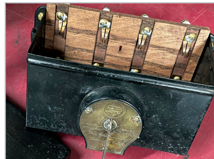
7) Rebuilt coil box with brass nameplate over switch
