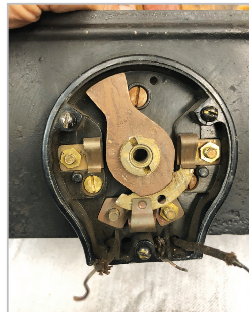
2) Remove the wires from the terminals and the three brass screws and nuts to lift the switch away from coil box
