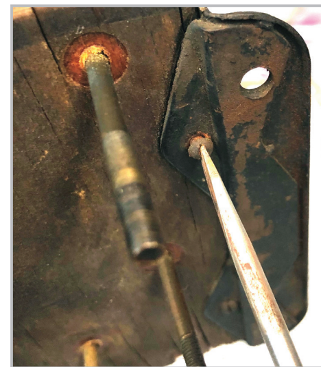
4) Remove wood screws to release back and base panels
