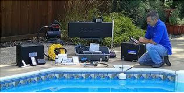
Once a leak determination is made then it is necessary locate the leak. Typically the leak types are plumbing or structural. Each requires *experience*, equipment and knowledge to detect. I utilize underground listening sonar, to locate and pinpoint a plumbing leaks usually within a 1 sq. ft. area.
