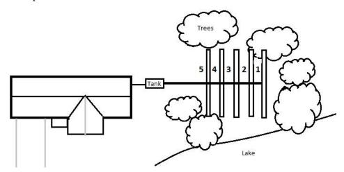
Above is an example of a multiple line installation. As you can see, the installation should begin with the line marked 1 and proceed to 2, 3 then 4. This procedure will greatly ease material handling and backfilling. (Note, sections of the drain lines should be left uncovered to allow for inspection of lines when area is confined and return access to lines is limited.)
