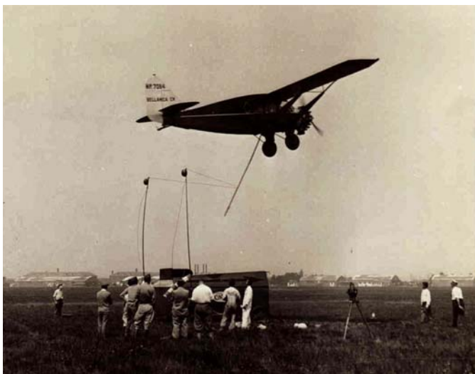
Figure 8. Demonstrating the new Cabot aerial pickup. Mail bags, fastened to long reed-like poles, with a cord between them, are picked up by an airplane going at full speed. The plane is being piloted by Roger Wolfe Kahn.
