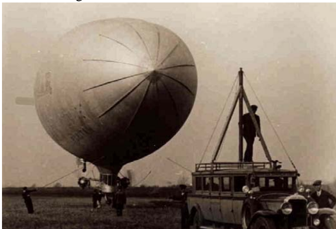
Figure 10. Bus acts as blimp's nurse. Portable mooring mast, mounted on bus, to speed up dirigible traffic, proves success in tests, bus racing airship off to fast start, also quick landing.
