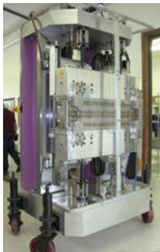
Figure 2: One meter wiggler insertion device for ALBA Synchrotron
