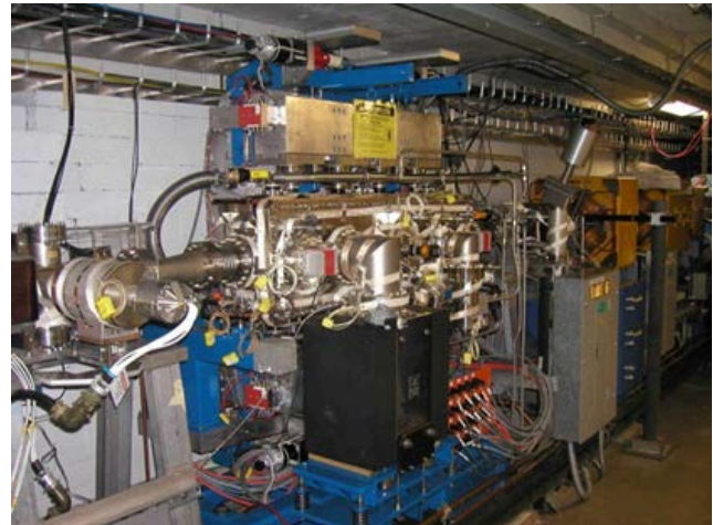
Figure 1: BNL Cryogenic cooled in-vacuum undulator in the ring
