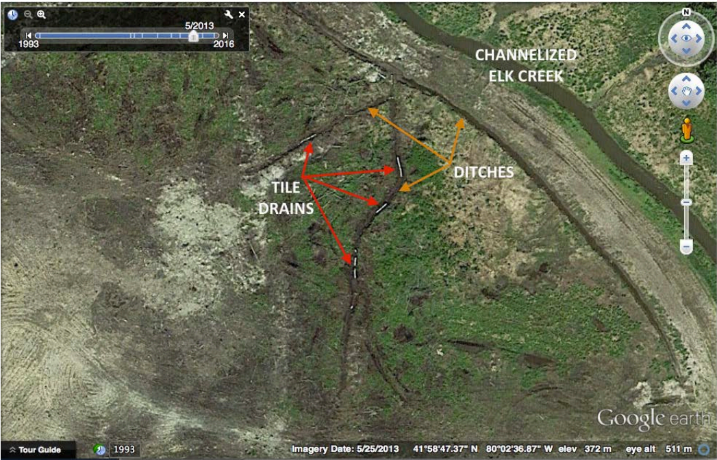
Figure 47 (close-up Figure 11). May 2013 aerial photograph of the Marsh Site (natural color, Google Earth) showing extensive disturbance of vegetation throughout site to bare soil, scattered logs and branches on the ground, plus labeled hydrologic alterations of tile drains (red arrows) and ditches (orange arrows) causing changes to wetlands in the floodplain of Elk Creek (near Sample Point #5).
