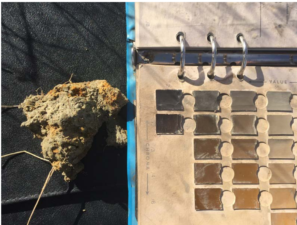
Figure 20. Munsell soil colors for Sample #1 showing hydric matrix, brighter mottles and oxidized rhizospheres (see text for discussion).
