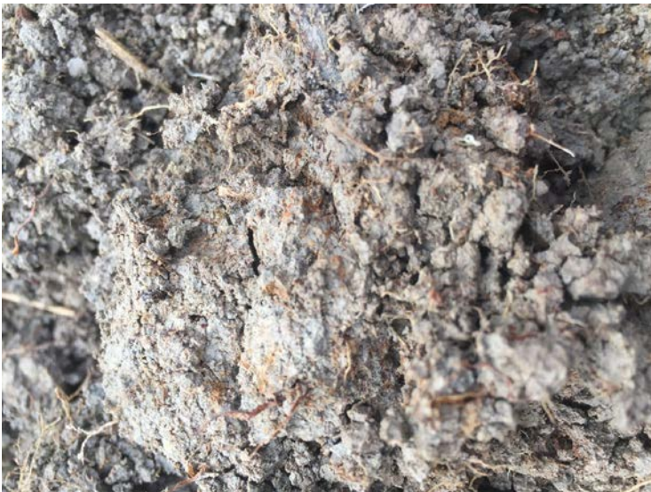
Figure 25. Marsh Site Sample #3 oxidized rhizospheres, 9-10 inches depth (see text for description).
