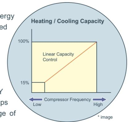
Using proven single inverter driven compressor technology, the CITY MULTI range is favored by the industry for low starting currents (only 8 amps for a 16HP YJM-A outdoor unit), and smooth transition across the range of compressor frequencies.
