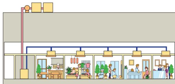
Water cooled systems can be used even in buildings that are taller than 50m by running a main water pipe through each floor.
