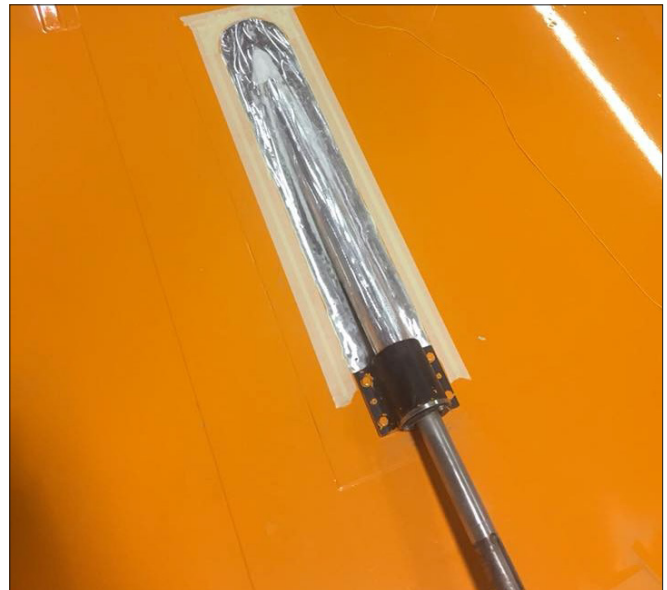
Shaft log installed
