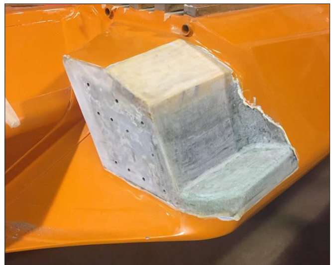
Skid fin bracket repair
