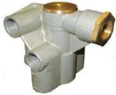
Spring Brake Control Valve - 4 Ports - Spring Brake Priority
