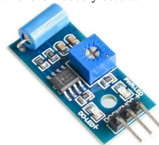
Fig.6 Vibration Sensor
