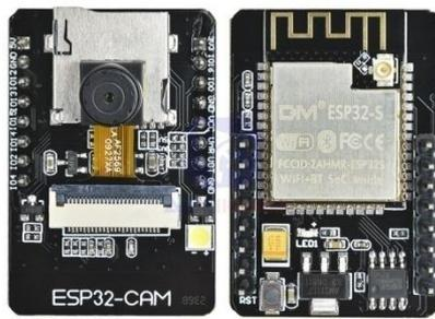
Fig.8 ESP32 camera
