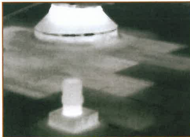
Photograph 1: Board stock anomaly of wet insulation in stair-stepped fashion.
