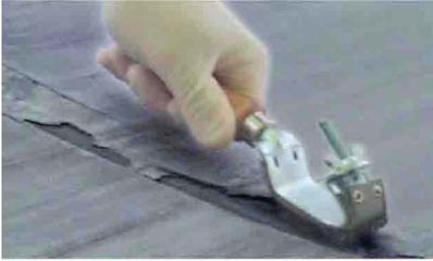
The conveyor belt or rubber surface must be clean, dry and rough. Use a stiff bristle wire brush or electric grinding disc (use slowest speed).
