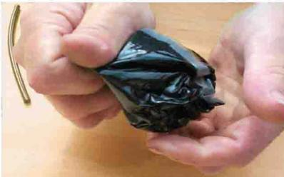
Mix by kneading and squashing the resin pack together until the Eli-Flex starts to warm up (3-4 minutes).
