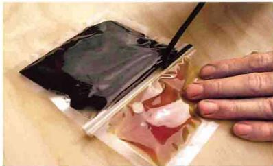
Once Eli-Flex pack is out of the foil sleeve, grasp both sides and gently pull apart until separator pops up. Slide out the separator and remove the divider clip.
