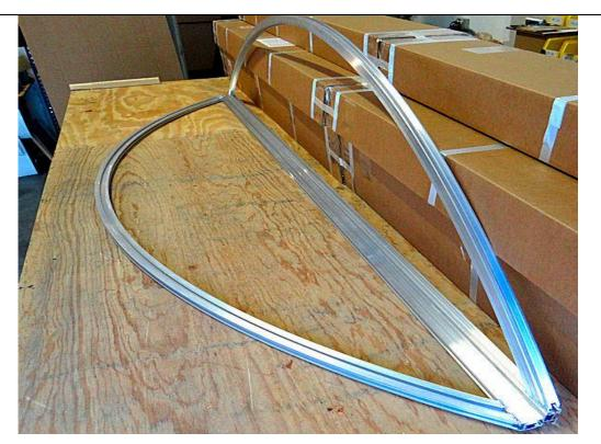
Here are the two tops for the two Arched Frames of this particular project, welded at the metal shop.
