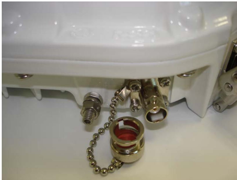
Figure 28 BNC Connector for RSSI Voltage
