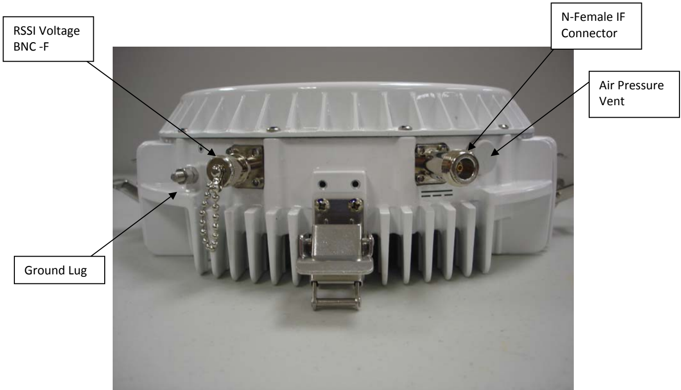
Figure 4 Outdoor Unit Connectors/Indicators (HP Model)
