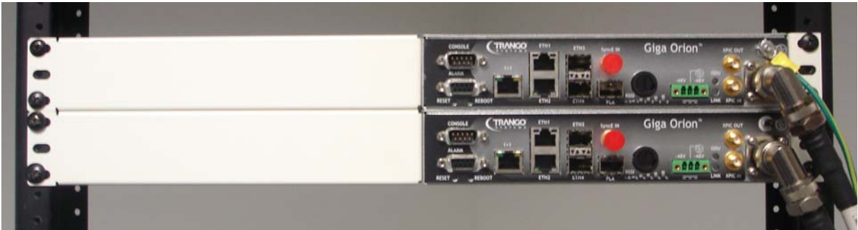
Figure 16 Mounted IDUs with Rack Ears installed
