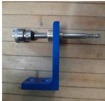
3. Re-attach L-Bracket to lathe base in appropriate holes with 5/32" Allen Wrench. Use hole setting that will that work best with the cartridge length you will be trimming. Use your best judgement to allow for room to work and full movement of driver. Don't worry the screws to reattach the L-Bracket are self-aligning!
