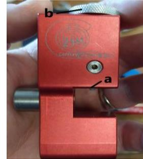
6. Attach cutting body to left L-bracket with tool body screw (A) with the two aluminum spacers (B) on screw on the inside of bracket as pictured. Tighten screw (A) with 5/32" Allen wrench so that the cutter body is tight against the L-Bracket and the spacers without any play. Note (Do not use the rubber flat washers that are used in the neck turning set-up) Do not over tighten.
