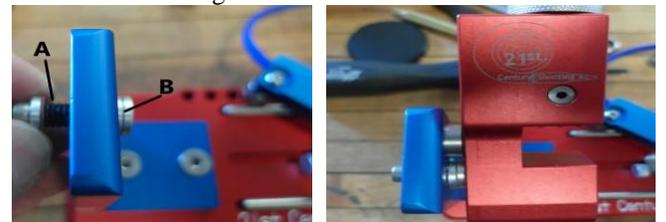
7. Cutter body should be at an angle where you can see the trimming operation. Roughly a 45 degree angle or more.
