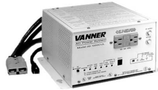
Vanner Charger/conditioner, transfer relay 20 amp KKK spec portable equipment charging circuit. Output is 1050-watts continuous, with a 2100-watt surge capacity.
