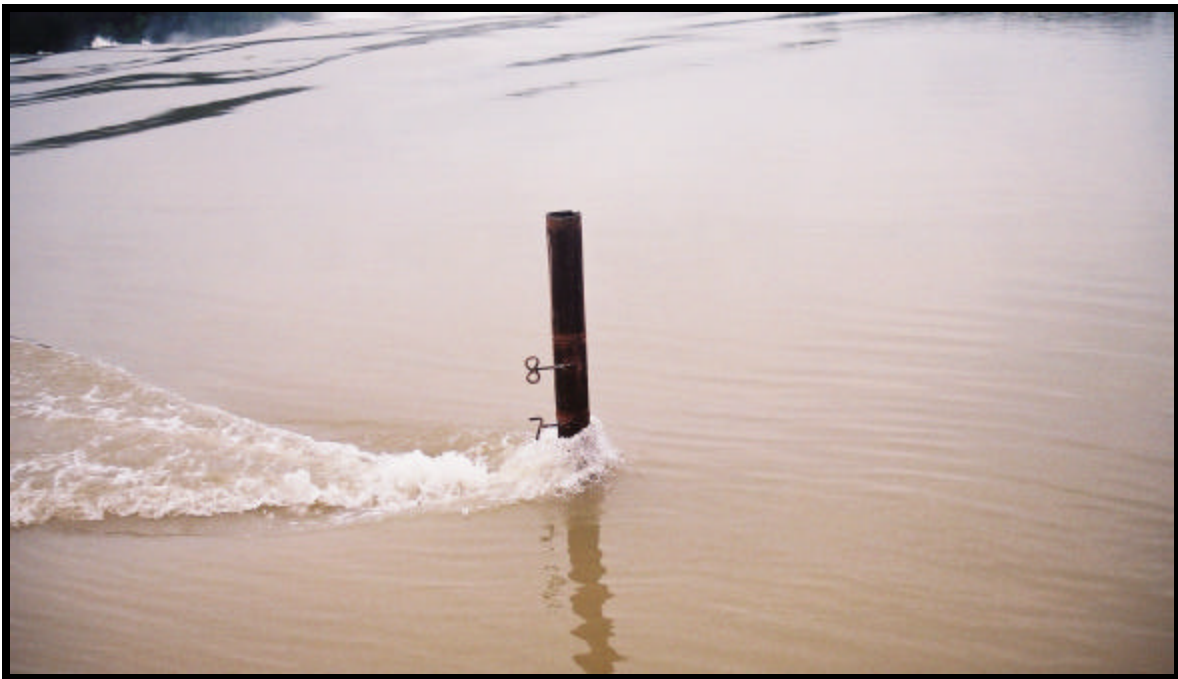
Photo 2 View of staff gage recording stage height (perhaps over the emergency spillway crest). The gage was located in the drawdown region upstream of the emergency spillway, as evidenced by the accelerated approaching flow and resulting standing wave around the gage. (Friday, July 5 th )
