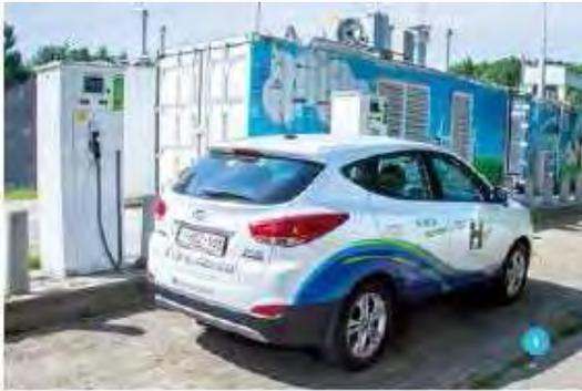
**A car can drive 100 km on 1 kg H<sub>2</sub>, while a bus can drive the same distance on 7-8 kg H<sub>2</sub>. Both typically travel 400-500 km before they need to refuel. A fuel cell car usually has a 5 kg tank at 700 bar, while a bus tank holds 35 kg H<sub>2</sub> at 350 bar.**
