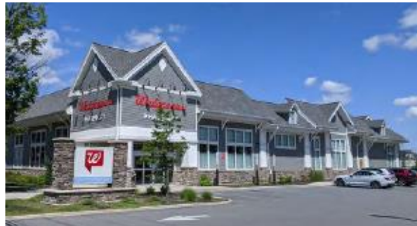
Figure 1318. This is an example of a franchise business with building design elements and signage that incorporates many of the design standards desired for the TC District. Note rooflines, lighting, signage, bollards, side parking, side entrance and windows.
