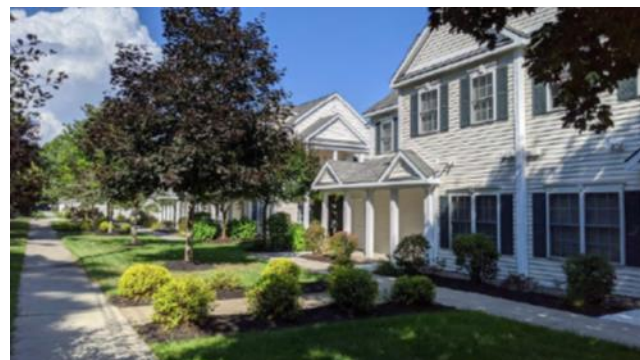
Figure 712. This multifamily development includes many design features consistent with the TC Design Standards including setbacks, sidewalks, front yard landscaping, traditional building styles, two story buildings, facade breaks, and traditional windows.
