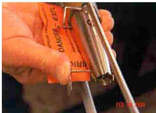
**Figure 6** Re-inserting the steel split pin into the Fuse Head before removing Penthrite Projectile from the Darting Gun.
