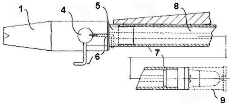
**Figure 15** The Body Assembly (broken) with propellant shell and part of barrel of the Darting Gun (striped). The Stirrup is shown both in "safe" position (unbroken line) and "armed" position (dotted line).
