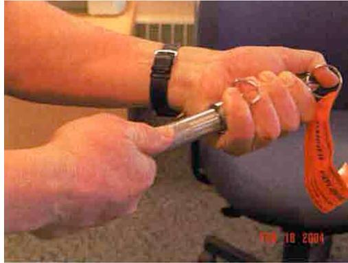
**Figure 10** Disassembling Fuse Head and Body.
