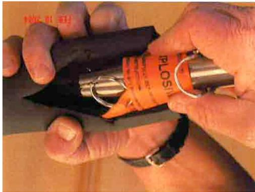
**Figure 12** Packing the Fuse Head in shock absorbing wrapping.
