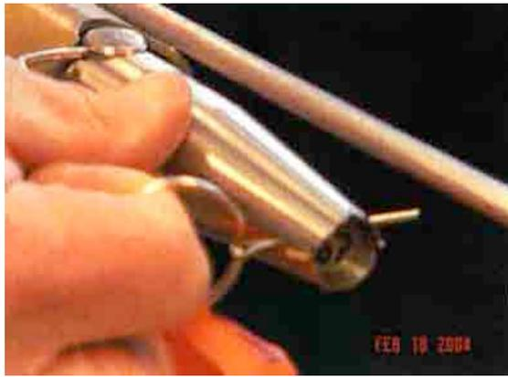
**Figure 5** The transport security steel split pin must be removed before the Darting Gun is thrown.
