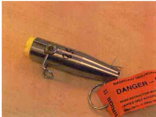
**Figure 16** The Penthrite Projectile mounted in the Darting Gun. The transport security steel split pin and the warning flag (note the extra split pin) are still attached.
