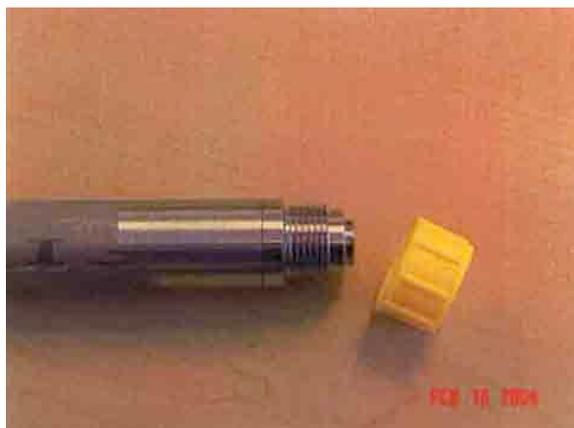
**Figure 19** The threaded connector for the Body and a plastic cap to protect the threads and the aluminum cap.
