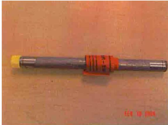
**Figure 18** Body of the Penthrite Projectile.
