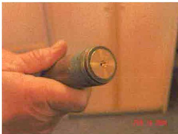
**Figure 4** To make sure the Projectile is secure against the wadding of the propellant shell, a blank shell can be used to check the fit.
