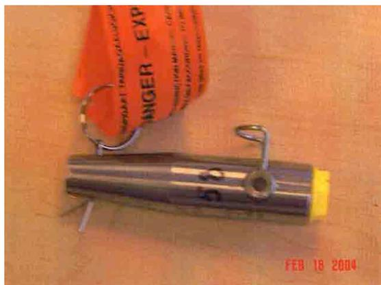
**Figure 13** Fuse Head with inserted transport security steel split pin and red warning flag (one steel split pin at the each end of the flag).
