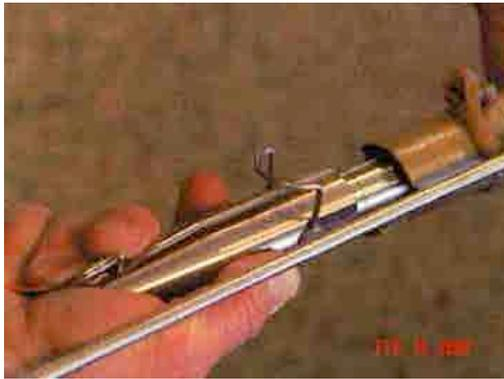
**Figure 7** Separating barrel and Darting Gun.
