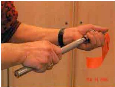
**Figure 2** Assembling the Body and Fuse Head of the Penthrite Projectile.
