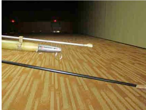
8. Keeping clear of the front of the barrel, place the Projectile Body in the Darting Gun barrel, with the "Stirrup" resting in its seat. When the Projectile is positioned correctly in the barrel, the washer will be seated firmly against the wadding of the propellant shell (Figs 4 and 5).
