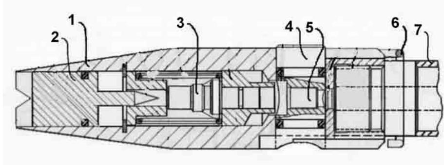
**Figure 14** Fuse Head Assembly of Penthrite Projectile (longitudinal section view).
