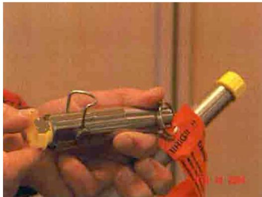
**Figure 17** Removing the plastic plug from the Fuse Head.
