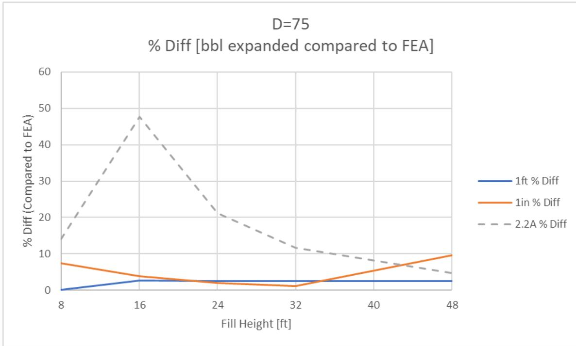
Figure 8 Volume Expansion at Various Fill Height (D=75)
