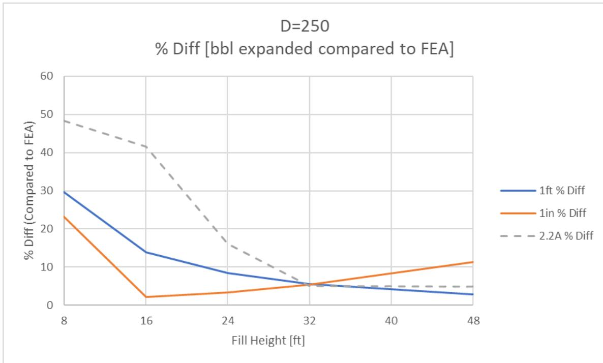
Figure 9 Volume Expansion at Various Fill Height (D=250)
