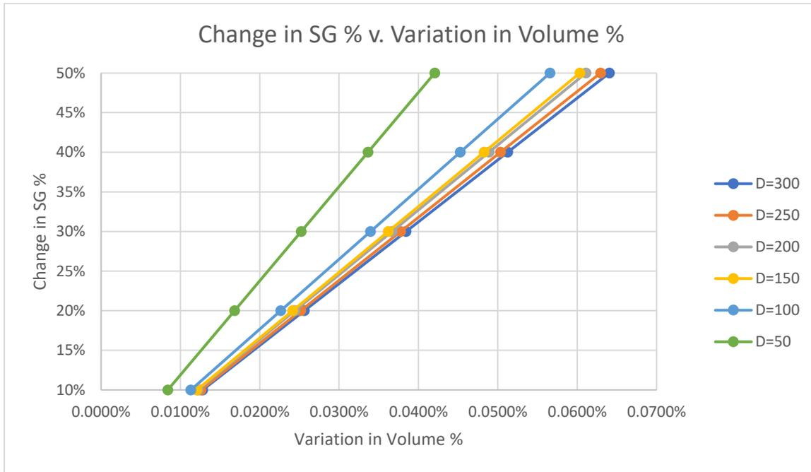
Figure 12 Volume Expansion for Change in SG (Diameters 50-ft to 300-ft)
