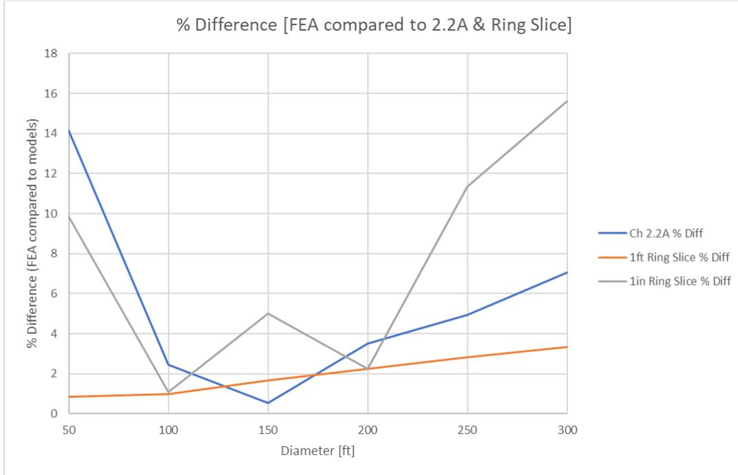
Figure 5 Percent Difference between FEA (ideal model) and Proposed Models (RSM & 2.2A)
