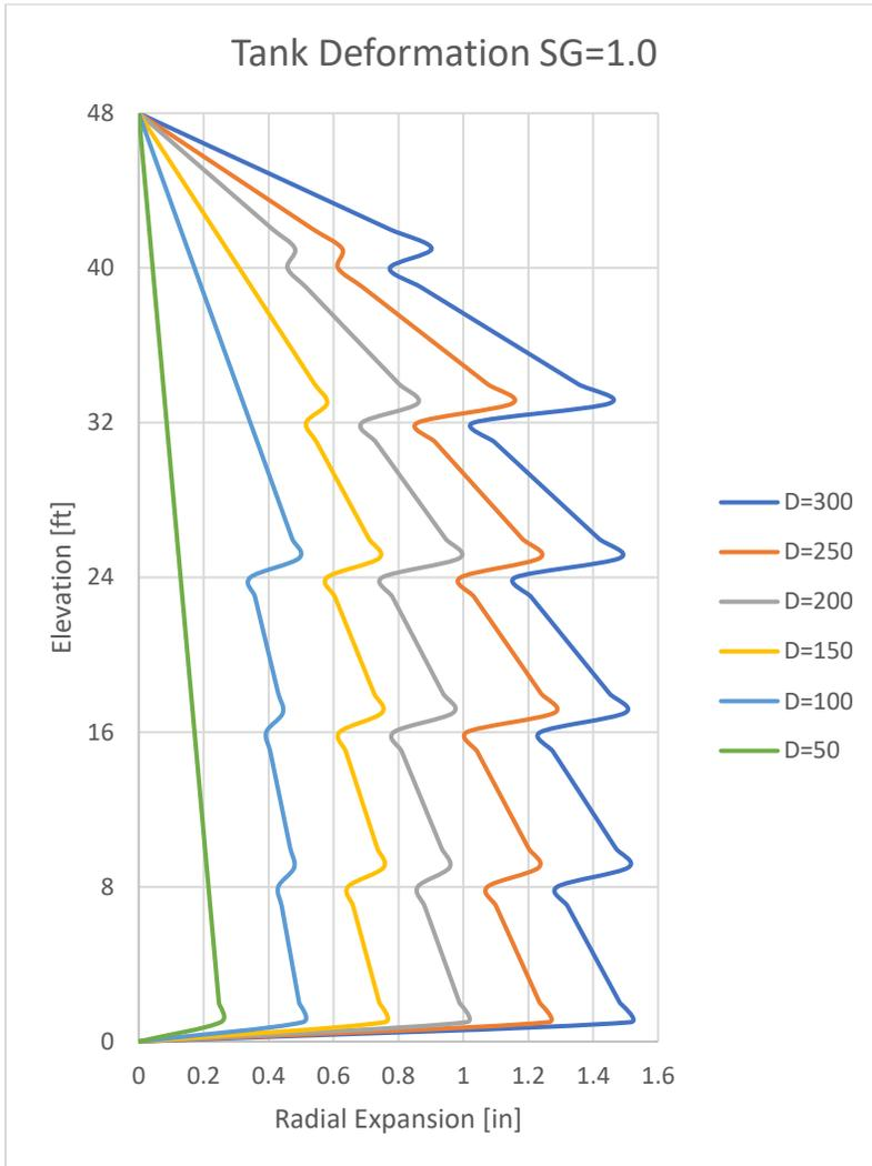
Figure 7 Ring Slice Method Radial Expansion for Varying Tank Diameters (SG=1.0)
