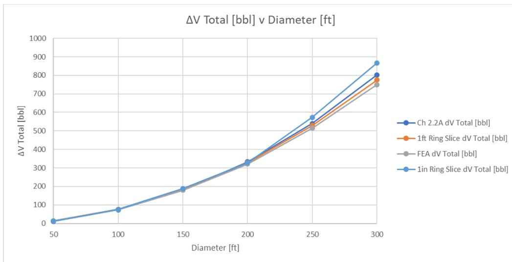
Figure 4 Total Volume Expansion for Varying Models of Diameters Ranging from 50-ft to 300-ft
