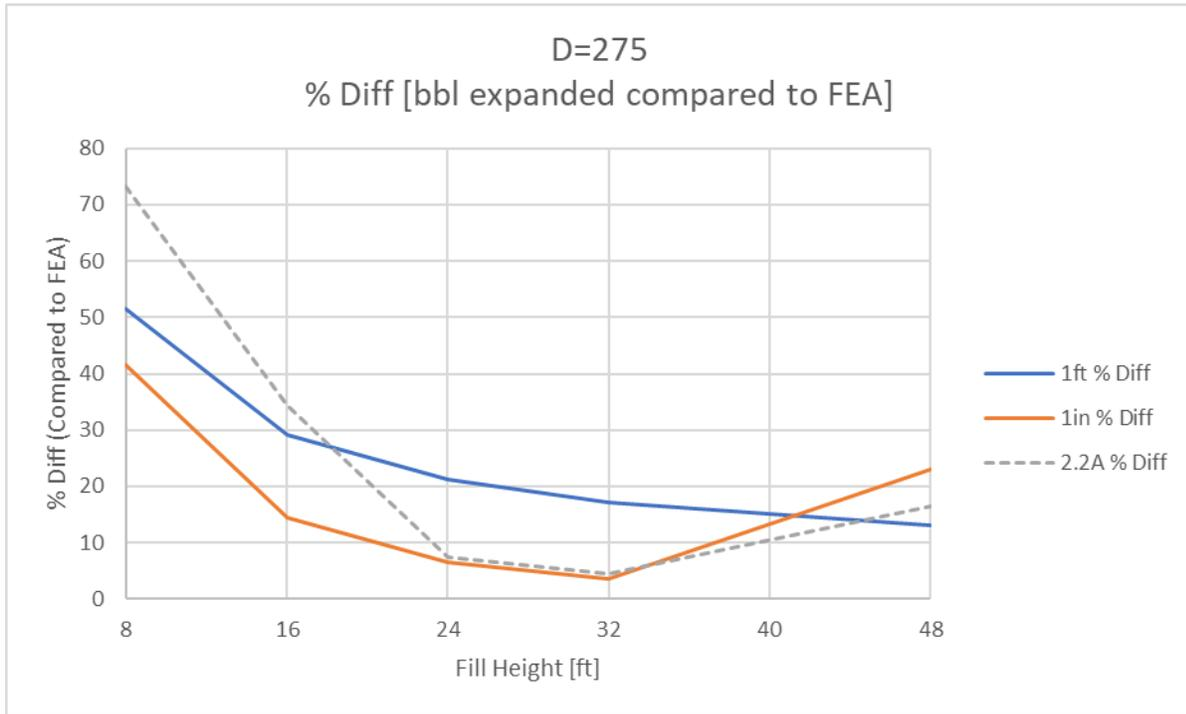
Figure 10 Volume Expansion at Various Fill Height (D=275)
