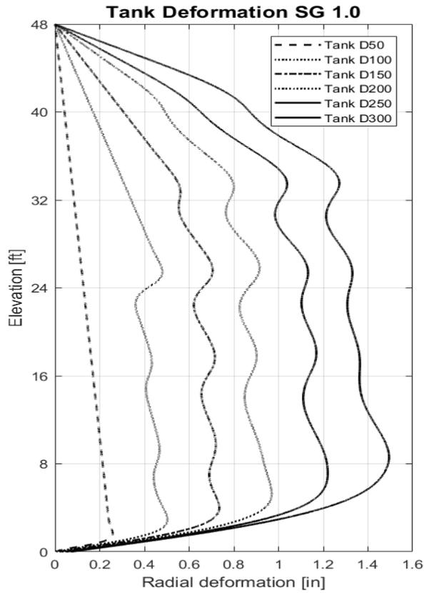
Figure 6 FEA Radial Expansion for Varying Tank Diameters (SG=1.0)
