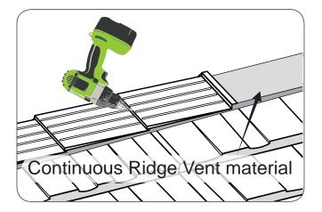
Cap fasteners to be 2-1/2"-inches in from the outside edge of the cap and installed through the nose of each cap, through the foam/seal-ant/ continuous ridge vent beneath & into the roof deck.
