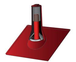
The Metro 3-in-1 SMART-jack is a moldable stonecoated roof flashing that can be used with most roof vent pipes, 1" to 3" in. (25-76mm) dia. Apply sealant under 3-in-1 SMART-jack for additional weather security.
