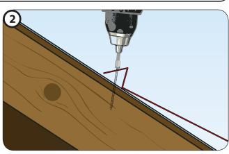
Panel back flange is 'seated' down onto roof deck.
