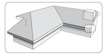
Metro Batten-less panels are installed on new or existing roofs pitched a minimum of 2-1/2:12 (12-degrees). Underlay is to be installed as per local code and manufacturer's instructions.
