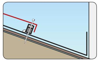
Position Metro SMART-XP-Foam or SMART-Barrier-Foam and fasten as shown above. NOTE: Metro Touch-Up Kits can be used to cosmetically coat the panel top fasteners, touch-up kit should not be used as the primary sealant.
