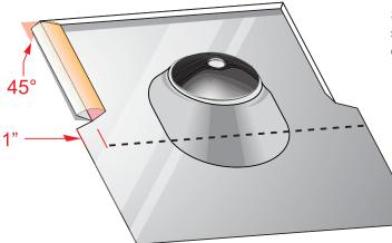
To prevent weather infiltration the edges of the SMART-Jack flashing should be folded/bent up as shown to channel any moisture onto the flashing and directed towards the lower panel.
