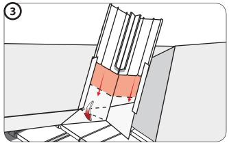
Install Valley metal over and onto the Stone-Coated Flat Stock.
