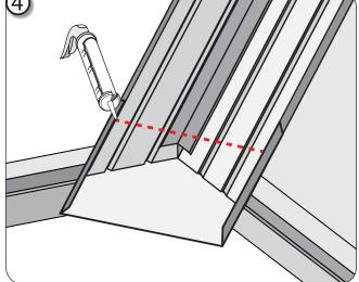
Apply a bead of sealant atop the Flatstock and seat the Valley Metal as shown.
