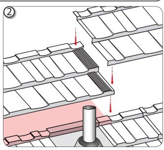
Install subsequent course above the SMART-jack flashing.
