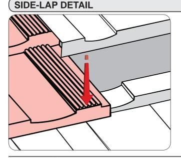
COTTAGE Shingle panels lay LEFT to RIGHT. Grooved right-hand side of the panel is the "Under-Lap" portion and is covered by the "Over-Lap" of the next full panel on the same row.
