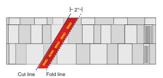
Measure, cut and fold up panels 2" (50mm) at the hip line. Install hip section panels similar to other panels placing additional fasteners through the up turned flanges as shown into hip board.
