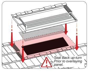
To prevent rodents and other vermin from entering attic space, the roof deck ventilation hole should be covered with 1/4" wire mesh.
