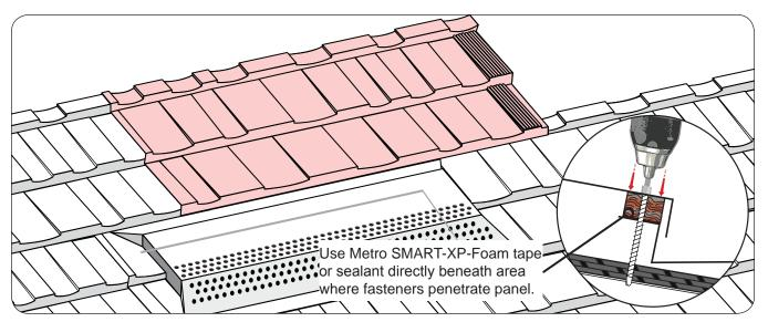
Top panel fastening is acceptable behind Metro SMART-Vents, Chimney's & Skylights as long as they are positioned out of the main water channels on the high ribs of the panel. Fasteners may be covered with material from a Metro Touch-Up Kit.
