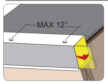
Install Drip Edge metal around entire roof perimeter, fasten per local code.
