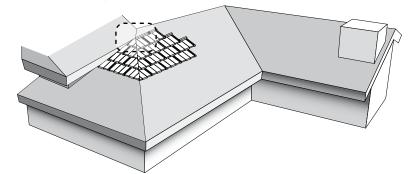
This is a critical roof area and requires special attention to ensure good weather protection. When the main roof intersects with a dormer roof, the panels back-lip where the valley exits onto the main roof must be flattened & the panels bent-up against the dormer roof, (See steps 1-4).
