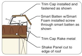
Metro Tile Rake Metal is installed along rake edges as shown. This rake edge metal aids in the alignment of Metro Trim Caps. The Metro Trim Caps install over the rake build-up and folded-up Metro panels.
