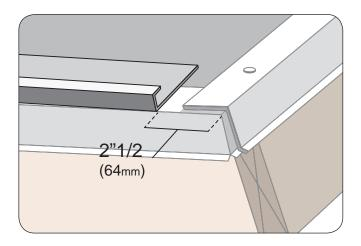
Use of Gutter Riser metal requires standard drip edge to be installed first. The Gutter-Riser metal is butted up to Rake Channel or Valley metal.
