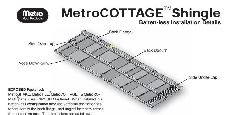
Overall Length Range: 52" (1321mm) Pitch (Course Cover): 14-1/2" (368mm) Side-Lap: 2" (50mm) Back Flange: 1" (25mm) Back Upturn: 1" (25mm) Front Nose Downturn: 1" (25mm) Panel Cover: 50" (1270mm) Panels Per Sq. (100-sq-ft): 20-pcs (0.465 panels per Sq M) Panels per pallet: 400pcs
