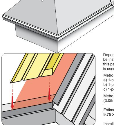
Depending on the valley metal used Metro panels can be installed to form either a 'Closed' or 'Open' valley. this page shows the Metro SMART-Valley metal which is used to create a 'Closed' valley.
