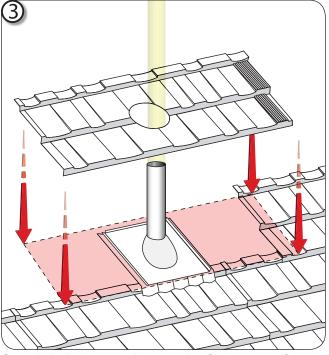
Cut a hole in the covering panel to fit the cone of the Pipe Flashing.
