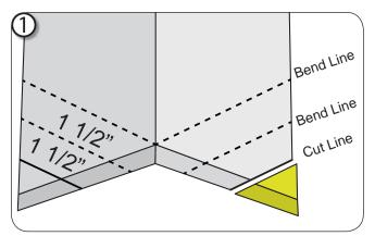
Mark cap as shown at center point. mark lines with 1 1/2" (38mm) of spacing.
