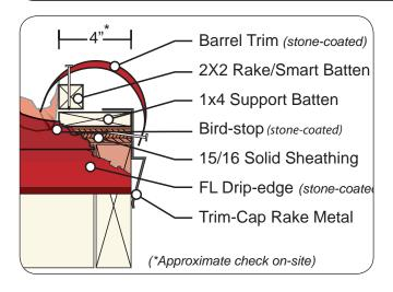
Metro Trim-Cap Rake Metal is installed along the rake edges as shown. This metal edging aids in positioning Metro Trim caps. Tile Rake metal is placed on the wood build-up. The Metro trim Caps cover battens and folded up Metro panel, as shown.
