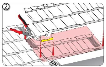
An alternative to folding panels up against walls, an "Under-Pan" metal can be installed next to the wall and behind an existing wall flashing. Metro Counter-Flashing metal or standard Z-Bar metal can be utilized to assist with weather-
