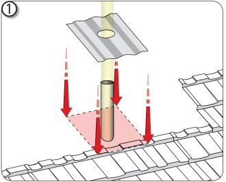
Cut 'Under-Pan' flashing around Vent Pipe as shown. Bend front edge of 'Under-Pan' over rear of under lapping panel.
