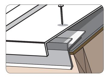
Fasten the First panel course up from the fascia through the top as shown. Top panel fastening is also acceptable behind Metro SMART-vents and chimney/ skylight details as nessesary.
