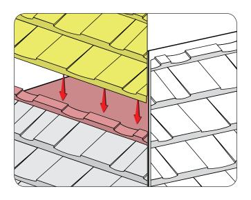
"Use the Metro SMART-Battens when installing Metro Shake 'V' Caps on Hips & Ridges."
