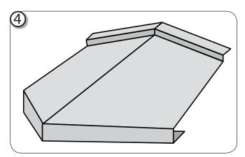
Fold Cap at the second bend line. Install Metro Smart-Barrier Foam (6" width) up the center. Install caps up the hip fastening each cap through the Smart-Barrier Foam to ensure weather protected detail.
