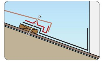
Use a V-Bat Riser Metal piece as shown to elevate the panel to the correct roof plane height. Fasten as shown with the panel nose being fastened into the V-Bat Riser.
