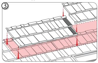
Apply either a bead of sealant or Metro SMART-XP-Foam or SMART-Barrier Foam along the top surface of the lower panel, just behind the dotted course line.
