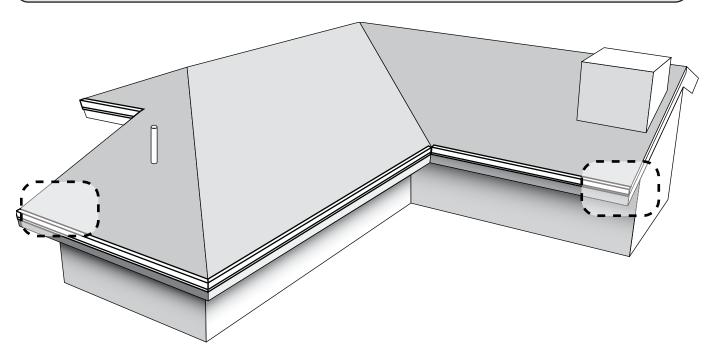
Install the Metro panels into the Rake Channel using fasteners placed as shown. If fasteners do not have a sealing washer, apply a bead of sealant around each one. Rake Channel metal is notched to lap a minimum of 2" (50mm) with water flow as shown. For other types of riser metals refer to the Optional details later in the manual.
