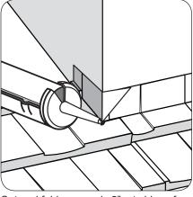
Cut and fold up panels 2" at sides of protrusion.
