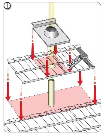
Cut a pipe sized hole in the covering panel. Install covering panel and apply a bead of sealant on each side and around the hole of the pipe as shown. Slide the SMART-Jack flashing over the pipe and seat it into the sealant. Conform the SMART-Jack Flashing to the panel contours.
