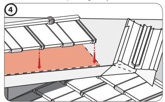
Then install the Panels regularly as valley cut out sections into the Smart Valley.
