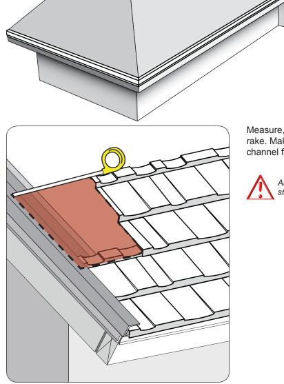
Measure, cut and install Rake panel sections up each rake. Make sure to insert each section into the rake channel fully.
