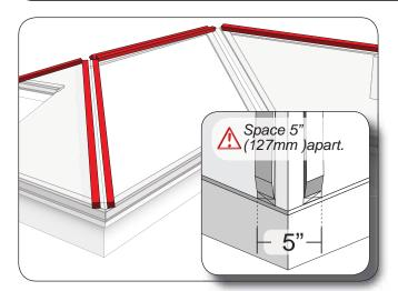
Metro panels are measured, marked, cut & bent-up approximately 2-inches (50mm) against the hip boards and fastened as field panels. The trim caps are then positioned over the upturned hip panel sections and fastened through each side of the hip caps into the hip boards.
