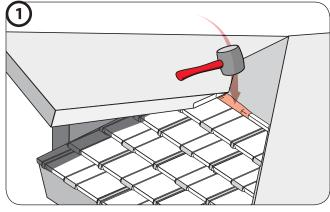
Flatten back flange against the roof deck.
