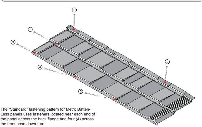
All fasteners used on a Metro roof shall meet or exceed the corrosion resistant standard as defined in ASTM B-117, (1,000hr minimum Salt Spray Corrosion Resistance).
