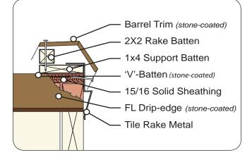
Metro Tile Rake Metal is installed along rake edges as shown. This rake edge metal aids in the alignment of Metro Trim Caps. The Metro Trim Caps install over the rake build-up and folded-up Metro panels.
