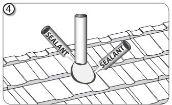
Seal Vent Pipe around bottom of cone and around pipe flashing as shown.
