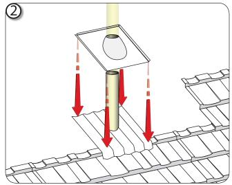
Install pipe flashing over 'Under-Pan'.
