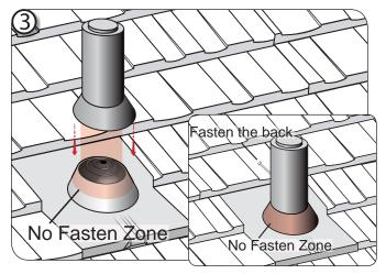
For added protection and appearance, SMARTsleeves are cut to conform to the panels and installed over pipes. SMART-sleeves are fastened with a screw through the back of the SMART-sleeve into the pipe.
