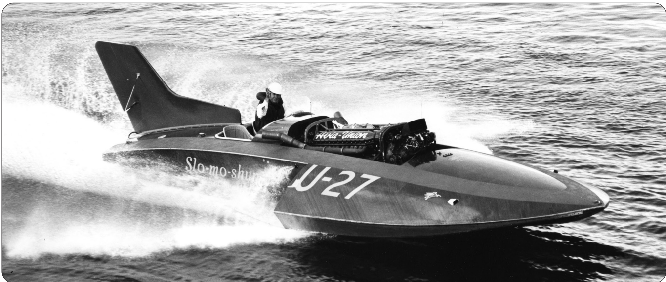
The “Grand Old Lady” Slo-mo-shun IV as it appeared in 1953. The boat’s most distinguishing feature that season was its mammoth Fiberlay tail, which was developed with the help of the Boeing Company to help counteract the impact of prop torque and provide better performance in the straightaways. Though it seemed to work, the tail was removed the following year in an effort to save weight.
