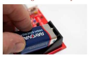
Example of how to insert the battery into the battery box at an angle, remember to do this with the power switch in the off position.
