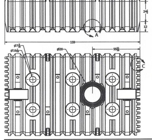
D Systems uses the largest capacity below ground storage tanks made today. Used to store water both potable and non-potable for a number of applications. The end ribs will accept fittings up to 4" in size. Integral columns in the tank give it excellent structural strength.
