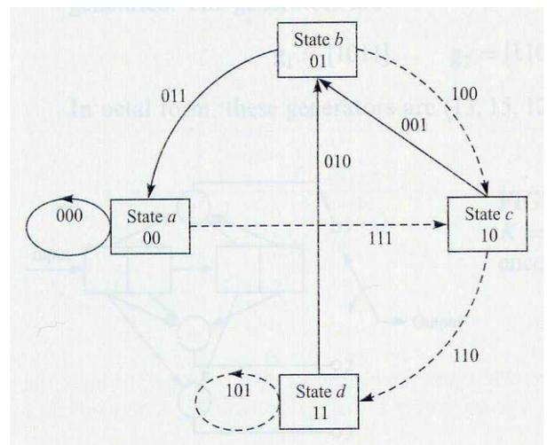
Fig.12: State diagram for rate 1/3, K=3 convolutional code.
