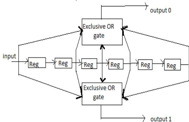
Fig.3: General Structure of shift register
