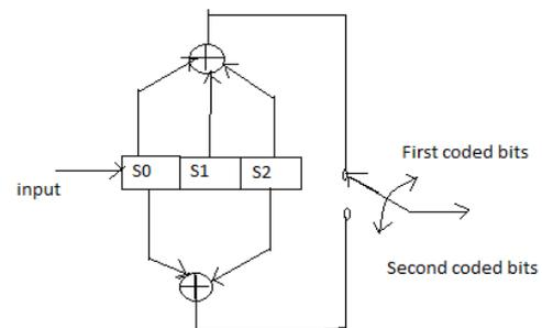
Fig.5: Rate 1/2 Convolutional Encoder
