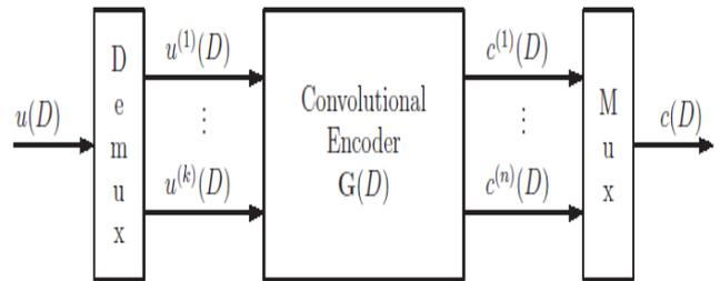
Fig.4: General Structure of Convolution encoder
