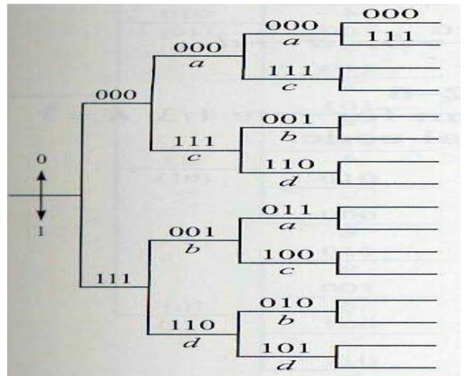
Fig.11: Tree diagram for rate 1/3, K=3 convolutional code.
