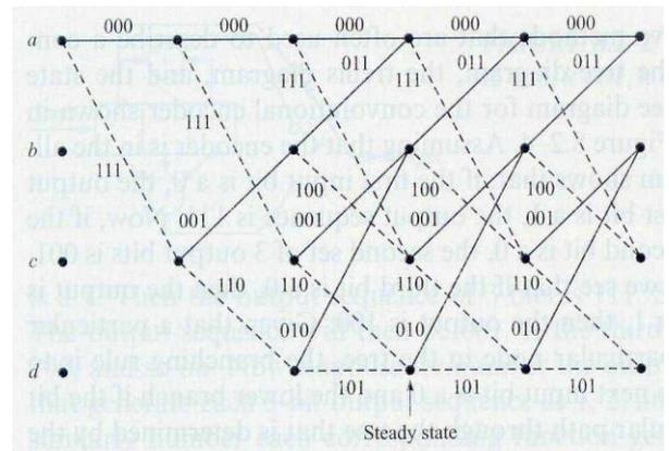
Fig.15: Tree diagram for rate 1/3, K=3 convolutional code.
