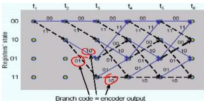
Fig.14: Tree diagram for rate 1/2, K=3 convolutional code.
