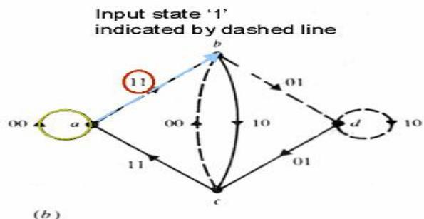
Fig.7: State diagram for 1/2 Convolutional Encoder
