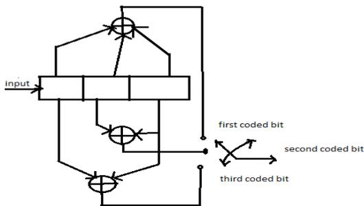
Fig.10: Rate 1/3 Convolutional Encoder
