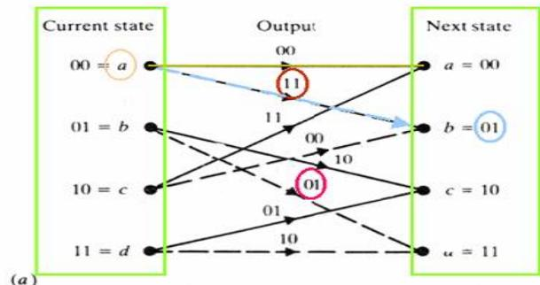
Fig.6: Trellis diagram for 1/2 Convolutional Encoder
