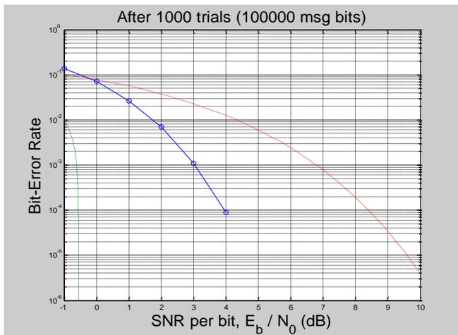
Fig.17: Simulated result for Convolution code for BPSK Modulation scheme.
