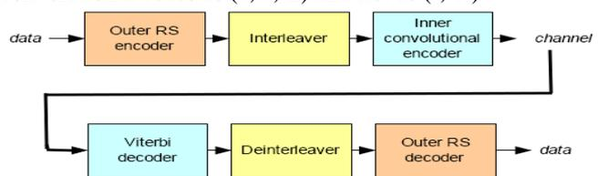
Fig.2: General block diagram for encoder and decoder
