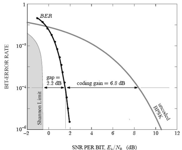
Fig.16: A simulated BER (log scale) versus  $E_b/N_0$  (in dB) curve highlighting both the gap to capacity with respect to Shannon Limit curve of a 1/3 system as well as the coding gain with regards to an un-coded code(Theoretical)
