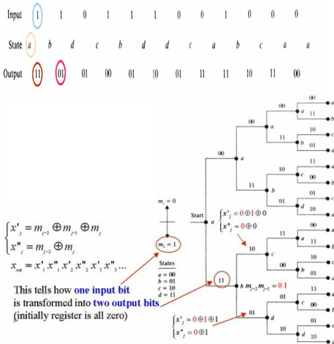
Fig.8: Tree diagram for 1/2 Convolutional Encoder
