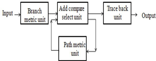
Fig.13: Block Diagram of Viterbi Decoder
