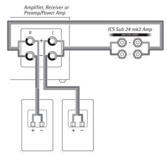
The other method is to connect the amplifier to the main speakers and then run extension wires from the main speakers to the ICS Sub 24 mk2.
