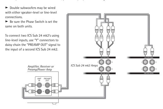
To connect two ICS Sub 24 mk2's using speaker-level inputs, use the "HIGH LEVEL INPUTS" binding posts on one sub-woofer to daisy chain to the second ICS Sub 24 mk2.
