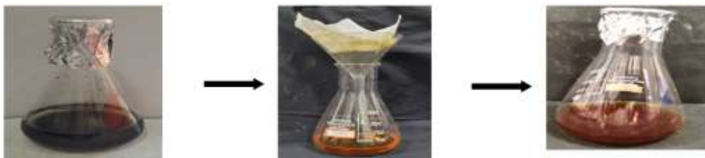
Fig. 4: Crude extract containing secondary metabolites which is obtained by means of ethanol extraction and subsequent solvent evaporation
