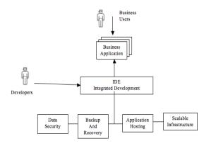
Fig.2: The concept of Platform-as-a-Service.
