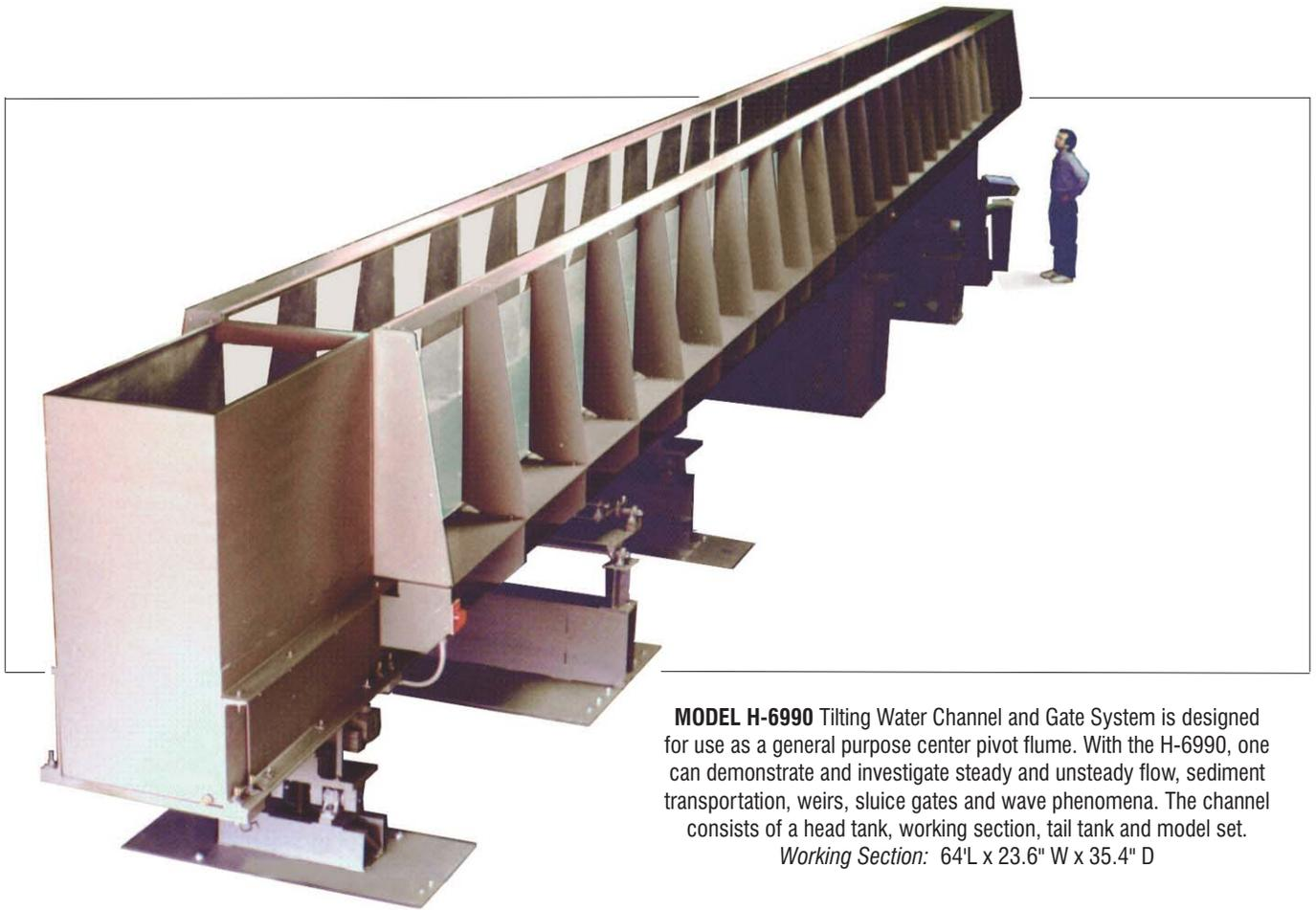
**MODEL H-6990** Tilting Water Channel and Gate System is designed for use as a general purpose center pivot flume. With the H-6990, one can demonstrate and investigate steady and unsteady flow, sediment transportation, weirs, sluice gates and wave phenomena. The channel consists of a head tank, working section, tail tank and model set.
