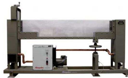
**MODEL H-6523A** Sediment Transport Demonstrator is designed to investigate suspended sediment in a moving stream and bed load movement. Simulates fast flowing streams or slow moving rivers to demonstrate the various sizes and densities of partial deposits. 0-10% slope.
