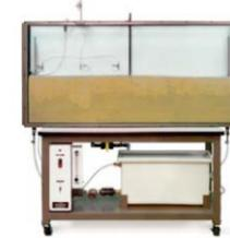
**H-6510** Drainage and Seepage Tank demonstrates water flow through permeable media (sand). Two-dimensional model flow lines can be determined as well as distribution of up-lift pressure and seepage rates.
