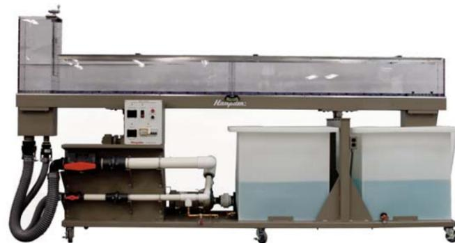
**MODEL H-6530** Mobile Hydraulic Demonstration Channel is designed for the investigation of analytical applications of fluid mechanics within a continuous media including conservation of mass, continuity, energy, and momentum. Application of these laws may be simplified in order to describe quantitatively the behavior of the fluid.
