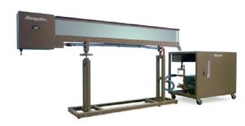
MODEL H-6940 Multi-Purpose Flume has been developed to investigate basic principles of fluid mechanics—various weirs, flume, gate syphon and spilling. Clear channel, inlet tank, discharge tank, pivot leg assembly, slope adjustment, pipe and flowmeter assembly and model set.
