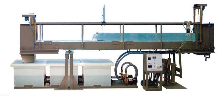
Hampden **MODEL H-6531** Hydraulic Demonstration Channel has been designed to investigate advanced analytical applications of fluid mechanics to situations in which fluids can be treated as continuous media. The particular laws involved include conservation of mass, continuity, energy, and momentum. Application of these laws may be simplified in order to describe quantitatively the behavior of the fluid.
