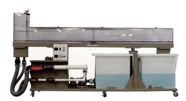
MODEL H-6530 Mobile Hydraulic Demonstration Channel is designed for the investigation of analytical applications of fluid mechanics within a continuous media including conservation of mass, continuity, energy, and momentum. Application of these laws may be simplified in order to describe quantitatively the behavior of the fluid.
