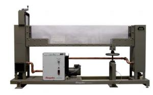
MODEL H-6523A Sediment Transport Demonstrator is designed to investigate suspended sediment in a moving stream and bed load movement. Simulates fast flowing streams or slow moving rivers to demonstrate the various sizes and densities of partial deposits. 0-10% slope.
