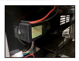
2. LOCATE IGNITER JUST INSIDE SIDE PANEL AND USING A METRIC HEX KEY REMOVE THE TWO SCREWS USING CARE NOT TO DAMAGE THE GROUND WIRE. REMOVE WIRES BY UNSNAPPING FROM WIRE TERMINAL.
