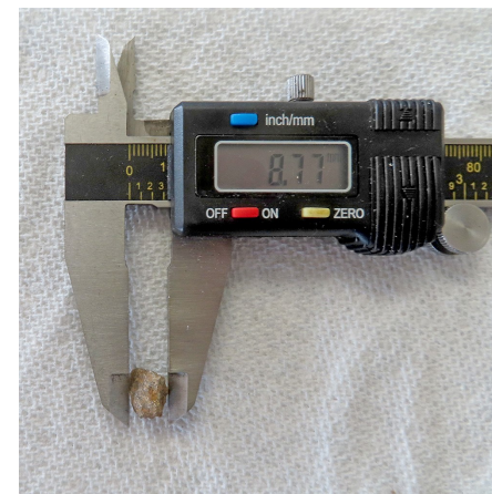
Using a digital caliper to measure average grain size.
