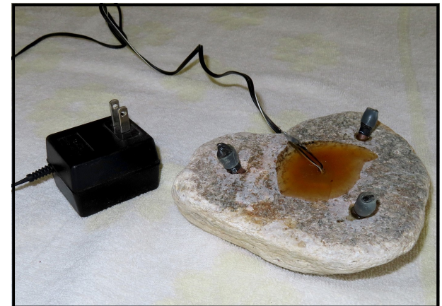
The bottom of the rock light showing the three metal legs covered with electrical shrink tubing, fiberglass resin sealing the LED, resistor, and electrical soldered connections, and the wall wart.
