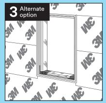
Weatherproof the installed wood buck with 3M<sup>™</sup> Ultra Conformable Flashing Tape 3015UC and 3M™ Air and Vapor Barrier 3015NP detailing tape. Ensure the tape is applied to prevent negative laps. The interior side of the wood buck should remain open, allowing it to dry to the interior if it would get damp.
