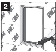
Install the bottom, then the sides, then the top and fasten per local wind load or building code requirements. Once all four sides are installed, apply sealant where the wood joins each other and around the entire perimeter.
