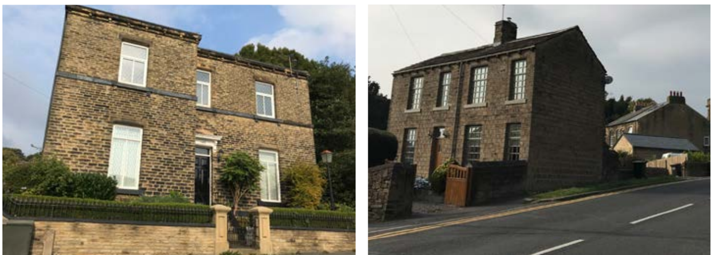
Figure 16: Photographs of building alignment to the street, usually either parallel to the street or set at 90° (often depending on topography and length of building). Working with the topography is often more efficient but stepped buildings also help to read the levels whilst providing 'eyes on the street'.
