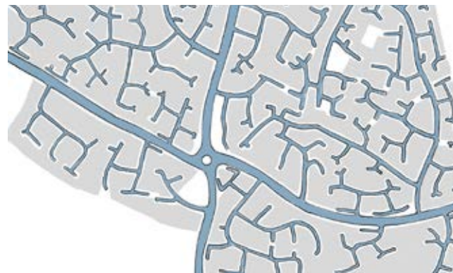
Figure 10: Example of poorly connected street pattern with cul-de-sacs with a limited hierarchy
