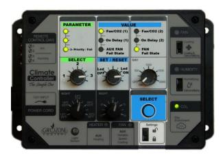
Ex. for FAN having priority over CO2 and FAN Fail State to OFF.
