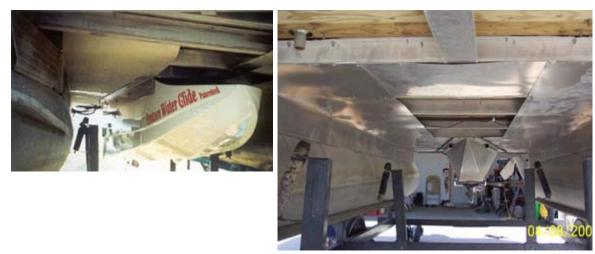
Install the 8' 4" x 2' aluminum sheets with 3/4" stainless steel self tapping screws that are provided in bag 2. Starting at the back of the boat, place performance sheeting to underneath side of floor joist / cross members and fasten with self tapping screws. (If you have existing sheeting at back of boat, start to overlap with new performance sheeting at that point.)
