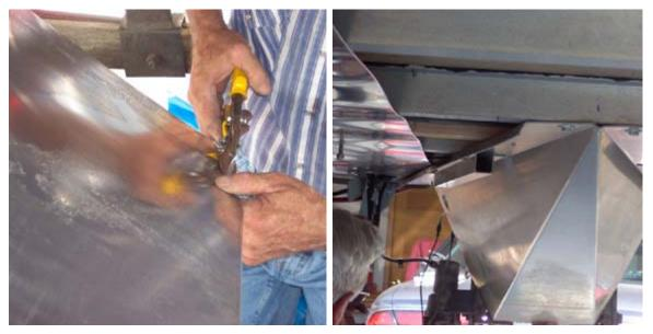
Overlap each sheet moving forward from back of boat decking so that your last sheet will stop at the desired floor joist / cross member. (DO NOT EXTEND SHEETING PAST FLOOR JOIST / CROSS MEMBER). The performance sheeting should run at least to the next floor joist / cross member past the front of the Water Glide.
