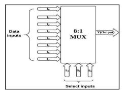
Figure 5.Block Diagram of 8\*1 Multiplexer
