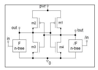
Figure 3.2N2N2P General Schematic
