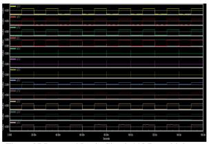
Figure 27.Proposed Logic Circuit 1\*8 Demultiplexer Output Waveform
