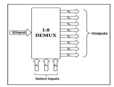
Figure 6.Block diagram of 1\*8 Demultiplexer
