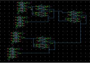
Figure 8.CMOS 8\*1 Multiplexer Schematic Design
