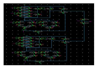
Figure 10.ECRL 8\*1 Multiplexer Schematic Design
