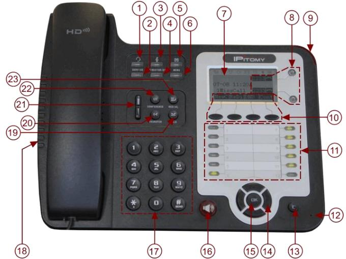
**Figure 4 IPitomy IP320 Buttons and Hardware Definitions**
